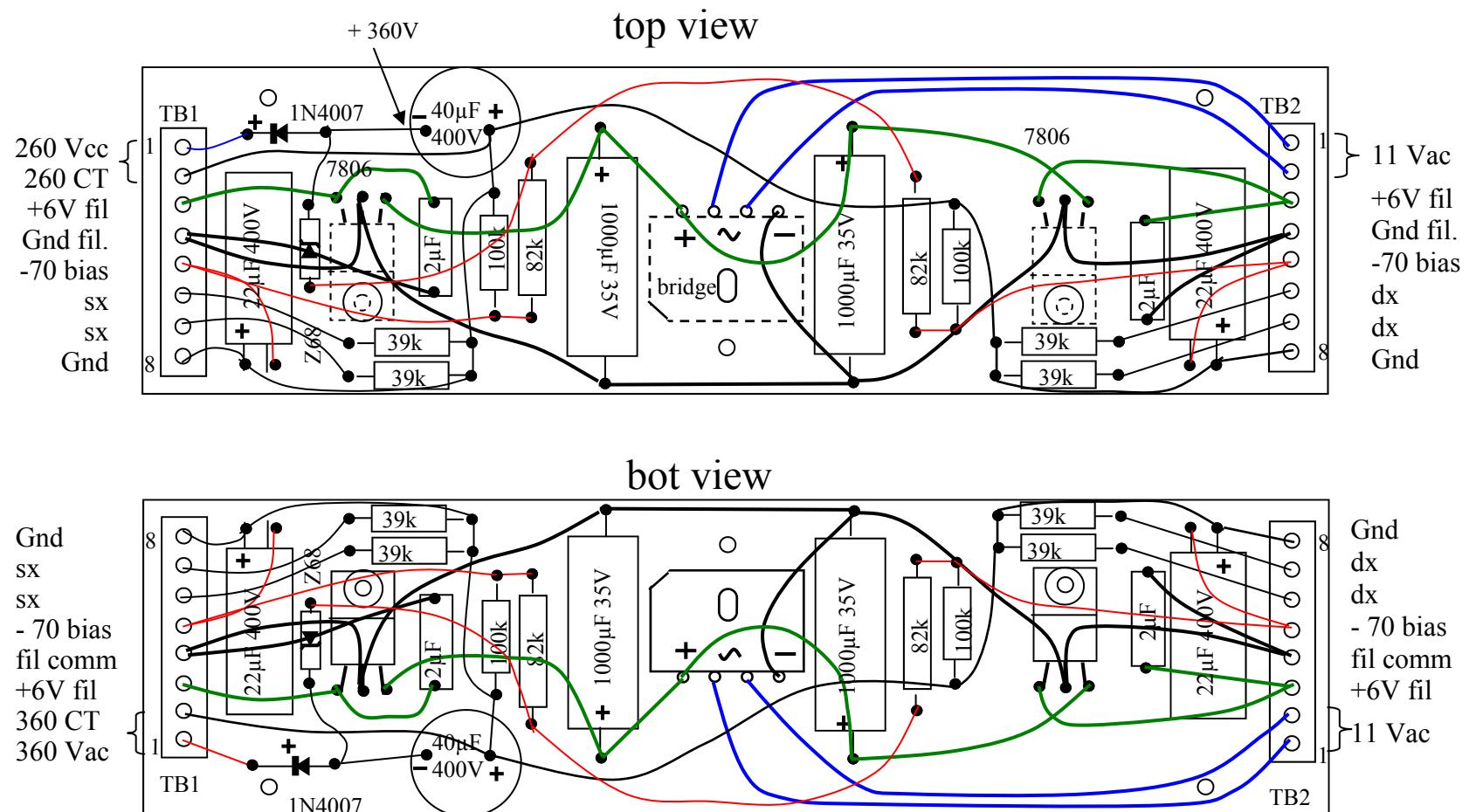
7806 IC and diodes bridge are mounted on the back side of board on an adequate heatsink
