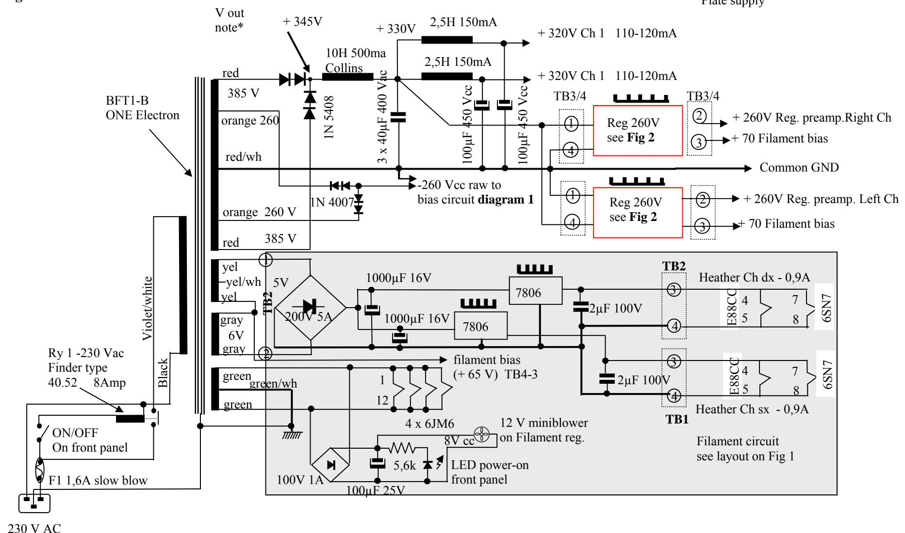
Fig 1 - 6JM6 bias voltage and 6SN7/E88CC DC filament layout
