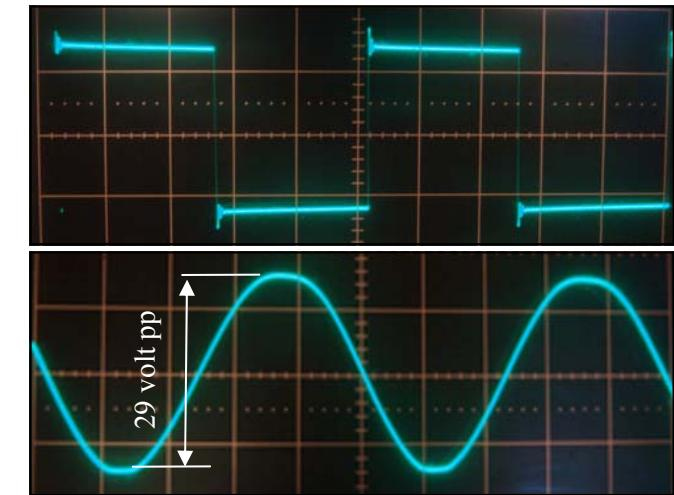
Top - Square wave 1 kHz 1W on resistive 8 Ohm load
