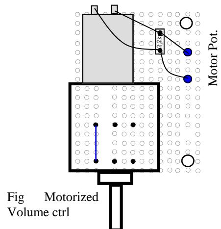
Fig Motorized Volume ctrl
