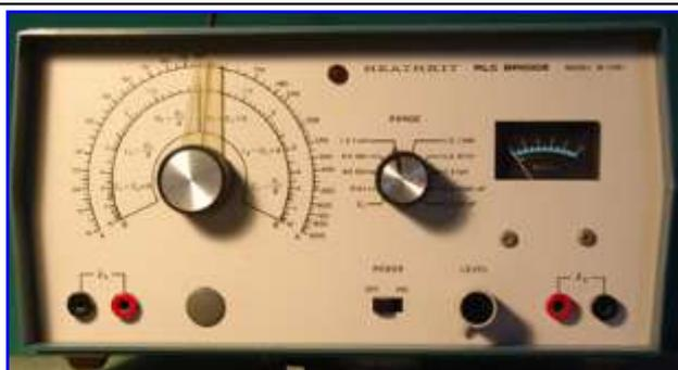
Ponte universale RLC HeathKit modello IB5281
